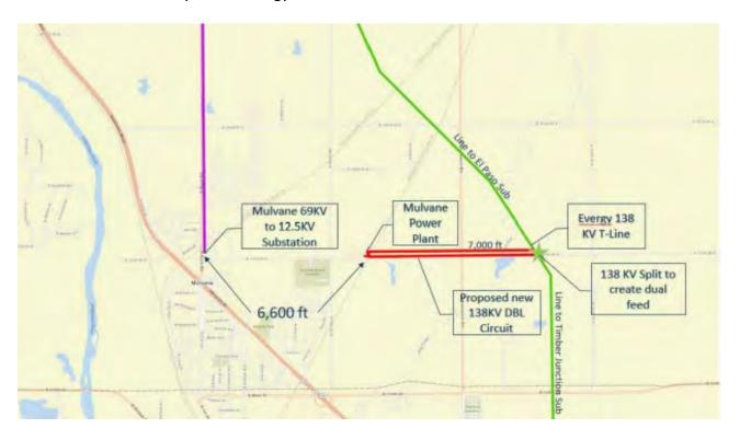
The project requires Evergy to build a new switching station to energize the city's new substation (proposed site layout below). Evergy is in the process of studying the site in advance of construction and is requesting a right of entry to effect the tests, surveys and studies related to construction of their infrastructure.
